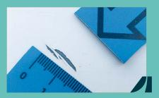
• Shallow grooves which do not penetrate down to the base paint and do not exceed 50 mm on any one body part.
