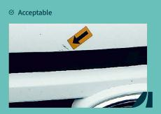
• Dents, bulges or other deformations up to a total of 100 mm per body part where the paintwork is not damaged.
