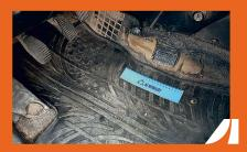
• Floor covering torn, areas which are worn through, burnt or excessively soiled.
