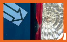
Holes, deep grooves, scuffed surface, cracks, broken off glass or plastic light cover regardless of size and quantity.
