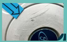
• Surface grooves, scratches, locally damaged paintwork.
