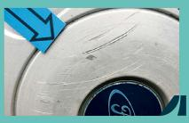
· Surface grooves, scratches, locally damaged paintwork.
