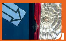
Holes, deep grooves, scuffed surface, cracks, broken off glass or plastic light cover regardless of size and quantity.
