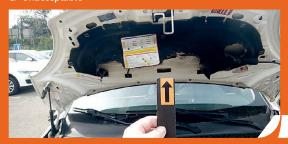
Damaged or torn soundproofing material on the engine cover or on the rear wall of the engine compartment.
