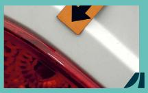
• Fine grooves, scratches on the surface, with no limitation of the functionality of the lights.
