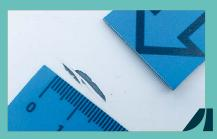
• Shallow grooves which do not penetrate down to the base paint and do not exceed 50 mm on any one body part.
