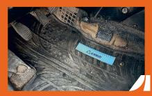
• Floor covering torn, areas which are worn through, burnt or excessively soiled.
