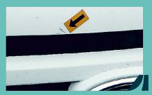
• Dents, bulges or other deformations up to a total of 100 mm per body part where the paintwork is not damaged.
