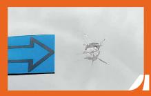
• Any damage which interferes with the driver's view or the structure of the glass.
